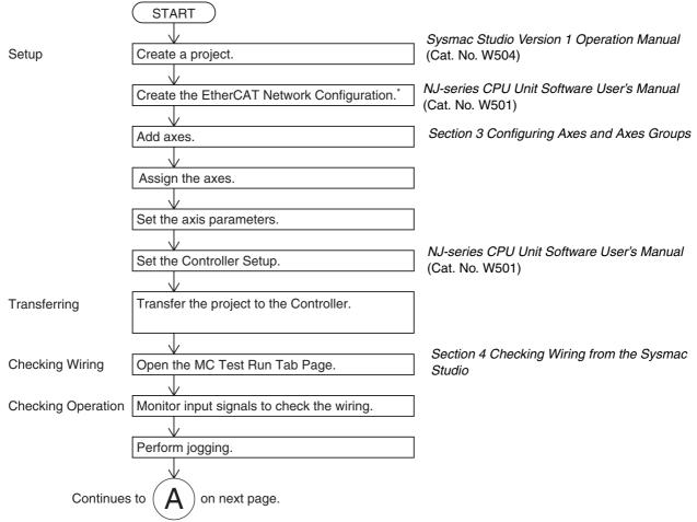
The EtherCAT Network Configuration can be set online if you are connected to the physical network. The EtherCAT Network Configuration can be selected offline if the hardware is not available yet.
