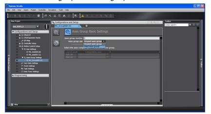
**3** Select the composition of the axes group in the *Composition* Box. A 2-axis composition is selected in the following example.
