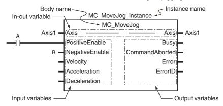
Specify the axis to jog with the *Axis* in-out variable. Change the *PositiveEnable* input variable to TRUE to start the axis with the specified positive *Velocity* (Target Velocity) and *Acceleration* (Acceleration Rate). Change *PositiveEnable* to FALSE to decelerate and stop the axis at the specified *Deceleration* (Deceleration Rate).
