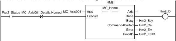
After home is defined for axis 0 and axis 1, the axes group is enabled.
