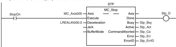
If the *Error* or *CommandAborted* output variable from the MC\_Stop instruction changes to TRUE, the MC\_ImmediateStop instruction is executed to stop immediately.
