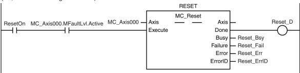
If the Failure output variable from the MC\_Reset instruction changes to TRUE, processing is performed to read the cause of the device error with GetFaultFactor. Program GetFaultFactor according to the device.
