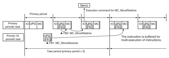
The values of output variables for a motion control instruction and the values of system-defined variables for motion control will change during the I/O refresh of the task that executed the instruction. Therefore, you may notice different behavior depending on the task if you use motion control instructions for the same axis in different tasks. Make sure that you thoroughly understand the processes of each task before you start to develop your user program.
