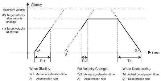
If you specify a short travel distance or a low acceleration/deceleration rate, the target velocity may not be reached. If the target position is exceeded after re-execution of the motion control instruction with the newly updated acceleration or deceleration rate, positioning is performed at an acceleration or deceleration rate that will enable stopping at the target position.
