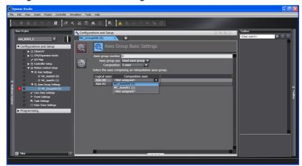
Click the bottom icon. The Axes Group Operation Settings Tab Page is displayed. Set appropriate values for the settings based on the operating conditions of the device.
