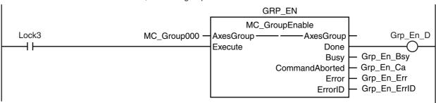
If there is a minor fault level error for the axes group, the axes group is disabled.
