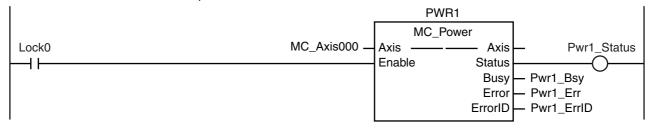
The Servo for axis 1 is turned ON if process data communications for axis 1 are active and normal.
