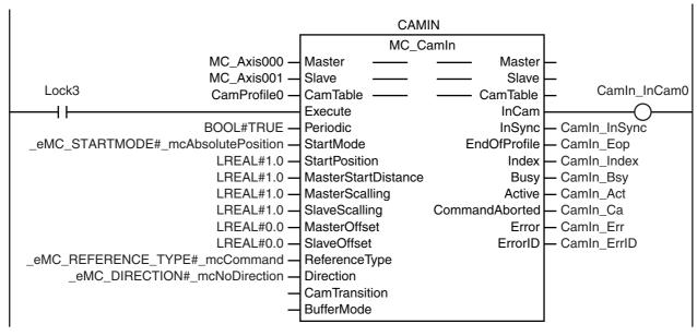
If CamTable1 is TRUE during absolute positioning, then the instance that uses CamProfile1 for the cam table is executed.
