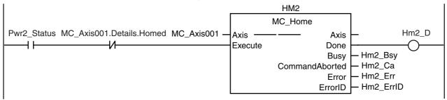
The status of the axes group and the status of home for axis 0 and axis 1 are checked.
