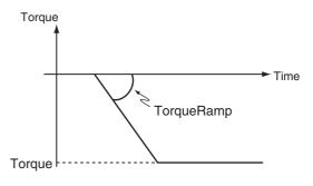
The MC Function Module uses the Torque Control Mode of the Servo Drive. The Servo Drive receives the torque command value from the MC Function Module in the torque control loop and to control the torque. You can specify the velocity limit value for the Servo Drive in the *Velocity* (Velocity Limit) input variable to the motion control instruction. You can use this to limit high-speed revolution of the motor when the load on the motor is low in Torque Control Mode.
