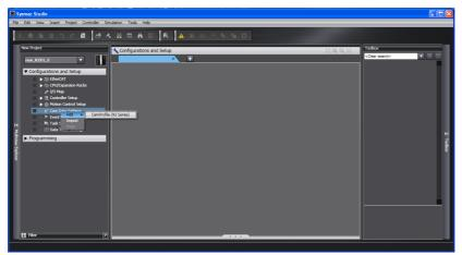
A cam profile is added to the Multiview Explorer. You can change the name of the cam profile as required from the default name of CamProfileO.
