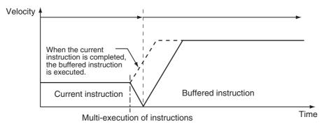
Use Rapid Acceleration/Deceleration (Here, BufferMode is set to blend with previous.)
