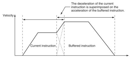
The output variable *Done*, which indicates the end of a motion control instruction, will change to TRUE for *TMCornerSuperimpose* when the area of superimposition is completed.
