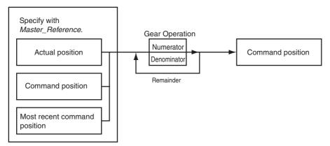
You can set the gear ratio numerator, gear ratio denominator, position type, acceleration rate, and deceleration rate for the slave axis to operate. For the master axis, you can specify the command position, actual position, or most recent command position.
