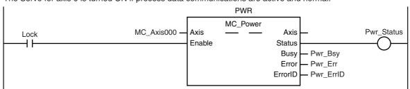
A check is made to see if any errors occurred when MC\_Power was executed before execution of further processing.
