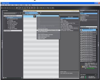
When obtaining the information is completed, the physical slave configuration of the EtherCAT slaves is displayed. Right-click the displayed physical configuration and select **Apply actual network configuration**.
