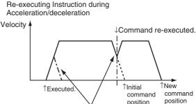
If you re-execute an instruction during triangular control or during deceleration, acceleration to the target velocity will occur again. This may result in a constant velocity.
