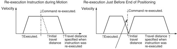
If the instruction is re-executed just before the end of positioning, positioning for the travel distance that is specified when the instruction is re-executed is sometimes based on the position to which the axis was moved for the initial travel distance.
