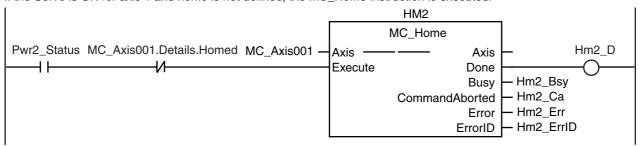
If homing is completed for axis 0, absolute positioning is executed.
