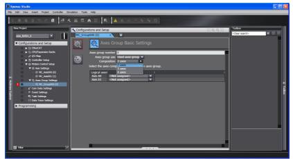
4 Assign the axis to use in the *Logical axes* Box.
