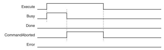
• The following timing chart is for when the input variable *Execute* is TRUE for only one period and an error does not occur for the instruction. The output variable *Done* will change to TRUE for only one period after the instruction operation is completed.
