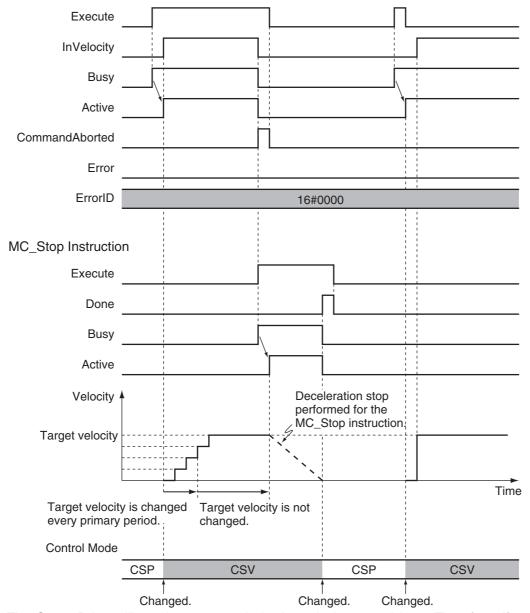
The Servo Drive will receive commands in the velocity control loop. Therefore, if any disturbance causes the velocity to decrease below the command velocity, no change in velocity will occur to remove the following error.
