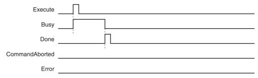
• The following timing chart is for when the input variable *Execute* is TRUE for only one period and an error occurs for the instruction. The output variable *Error* will remain TRUE.
