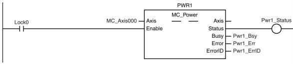
The Servo for axis 1 is turned ON if process data communications for axis 1 are active and normal.
