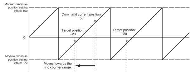
Similarly, the following example illustrates when the ring counter upper limit is 100, the lower limit is -70, the command current position is -20, and positioning is performed towards a target position of 290.
