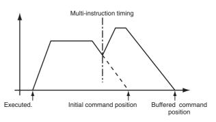
Multi-execution for axes groups is done so that the interpolation velocity remains continuous between instructions. If continuous operation is performed with an instruction with a travel distance of 0, the velocity changes for the axes will not be continuous.
