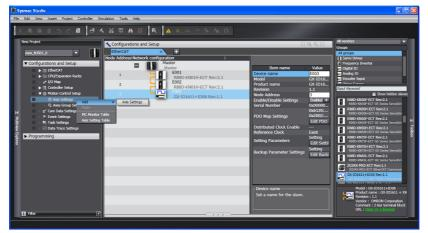
An axis is added to the Multiview Explorer. The default name for the new axis is MC\_Axis000.
