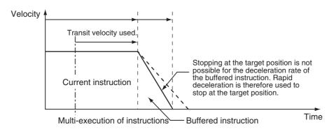
Use Rapid Acceleration/Deceleration (Here, BufferMode is set to blend with next.)
