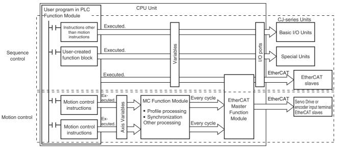
Normally, you must assign Axis Variables to EtherCAT slave Servo Drives. If you do not assign Axis Variables, assign device variables in the same way as for a general-purpose slave. Motion control instructions can be used in the primary periodic task and in a periodic task with an execution priority of 16 (i.e., a priority-16 periodic task).
