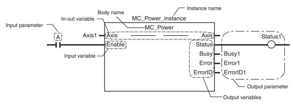
Specify the axis to move with the *Axis* in-out variable. Change the *Enable* input variable for MC\_Power to TRUE to turn ON the Servo. Change *Enable* to FALSE to turn OFF the Servo.
