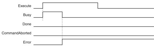
• The following timing chart is for when the instruction is interrupted during execution while input variable *Execute* is TRUE.
