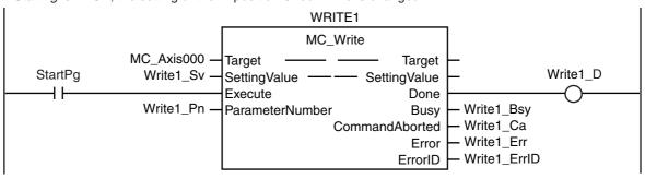
If changing the setting of the In-Position Check Time is completed, the setting of the Positive Software Limit is changed.
