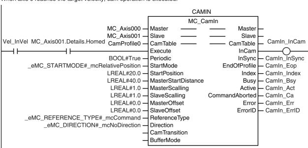
If StartOn is TRUE and cam motion is in sync, shifting the phase of the master axis is started.
