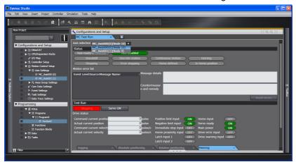
Check to see if the signals turn ON and OFF properly on the monitor screen by turning ON and OFF the sensor connected to each input signal.
