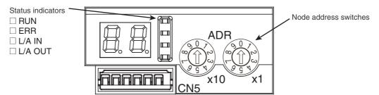
The rotary switches in the display area on the Servo Drive are used to set the EtherCAT node address.
